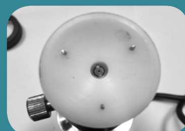
D) high brightness red LED (to illuminate the bottom of the eye)
